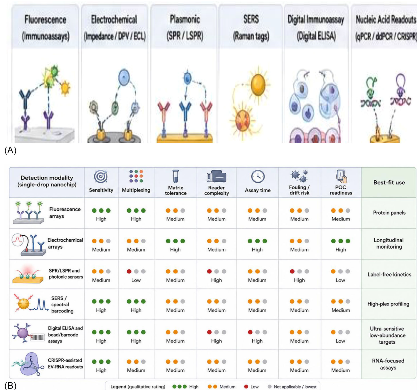
FIGURE 6 (A) Multiplex sensing architectures for exosome profiling. Detection performance depends on upstream exosome enrichment, sample matrix, lysis efficiency, fouling control, optical/electrical background, multiplexing burden and calibration stability under whole-blood or minimally processed plasma conditions. SERS, surface-enhanced Raman scattering; CRISPR, clustered regularly interspaced short palindromic repeats. (B) Performance trade-offs of exosome detection modalities under single-drop whole-blood conditions.
